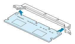
9 Push it firmly to make sure you fully insert the memory DIMM into the slot. The levers on each side are automatically latched.
